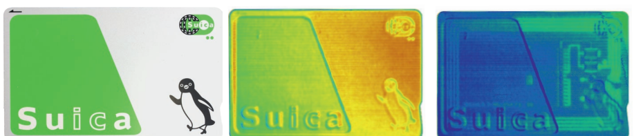
Photograph and terahertz images of a Japanese pre-paid public-transport card. The terahertz reflectivity image (middle) reproduces the look of the card. Removing the front-side reflection (right) provides an inside view of the underlying electronics.
