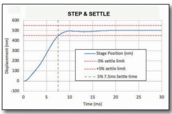
Settling time off the NanoScan OP400 stage with NPC-D-6110 controller with 150g load.
