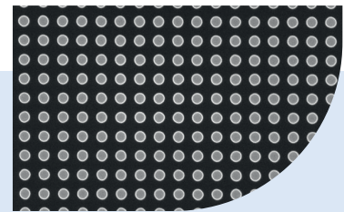
Square pillar array 300nm pitch
